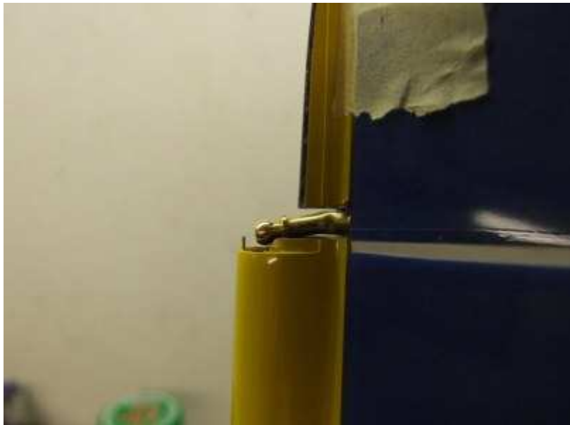
Glue horns with 5-min Epoxy. Side view should look like this (horns below hinge line).
