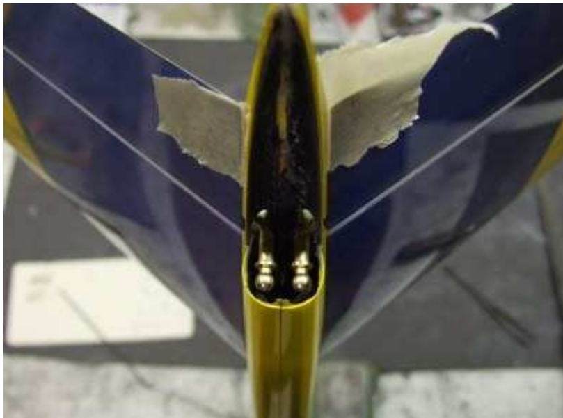
View from rear end. Flaps are fixed in neutral pos with tape.
