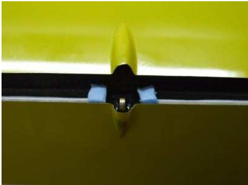
Glue horn with thickened epoxy.
